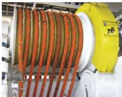
Quantum-8 turret buoy pull-in line installed on a traction winch on the FPSO Stybarrow.
