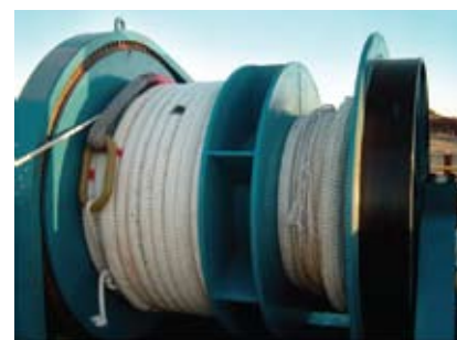
Tapered AmSteel®Blue with polyester jacket winch line, 60-mm diameter tapering to 44-mm diameter with master links spliced in.
